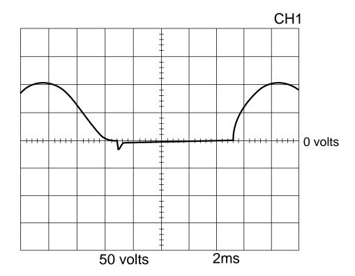
This is NOT the typical AC output voltage waveform. One output SCR is not functioning. Note the "gap" in the waveform. One SCR gate was disconnected to simulate an open or non-functioning output SCR. Each vertical division represents 50 volts and each horizontal division represents 2 milliseconds in time.
